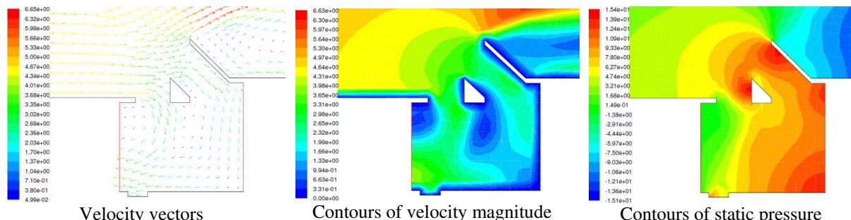
Fig. 24 Contours of velocity magnitude and velocity vectors in 5th composed intervention
