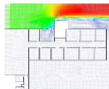
Fig. 7 Velocity vectors around the school (aisle window: close)
