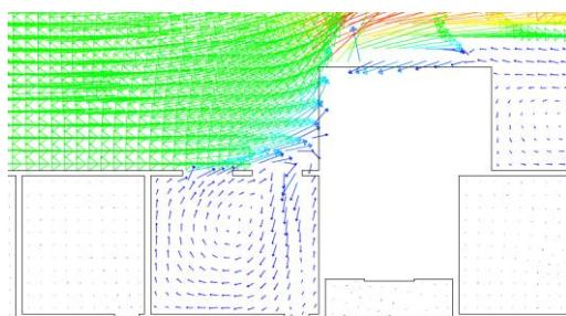
Fig. 8 Eddy current in case study (aisle window: close)
