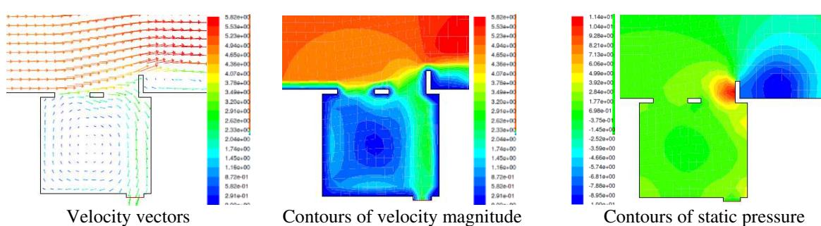
Fig. 13 Contours of velocity magnitude and velocity vectors in third intervention
