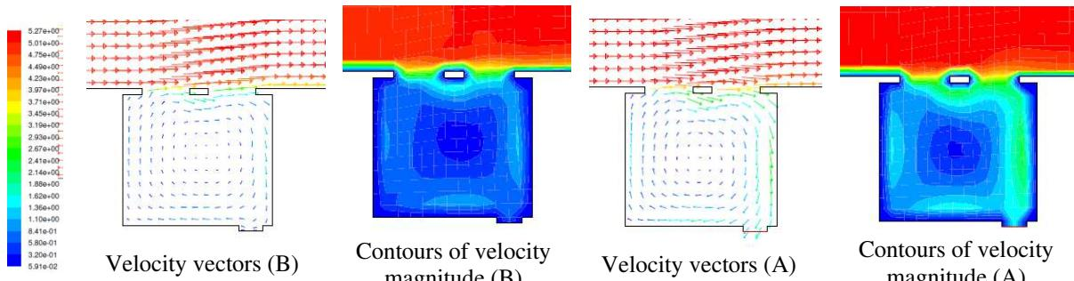
Fig. 11 Contours of velocity magnitude and velocity vectors in first intervention. A: the door is open, B: the door is close
