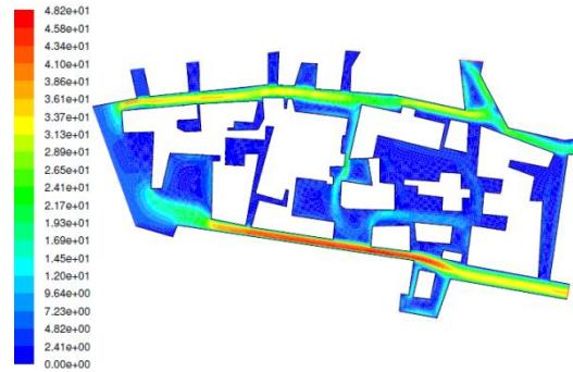
Fig. 4 Contours of velocity magnitude around the school
