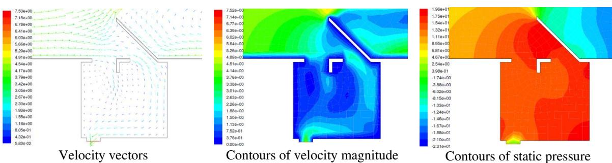
Fig. 21 Contours of velocity magnitude and velocity vectors in 2th composed intervention.
