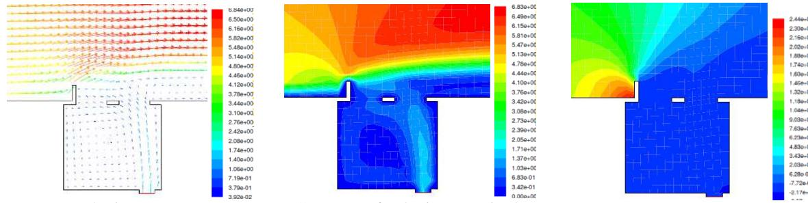
Fig. 15 Contours of velocity magnitude and velocity vectors in 5th intervention
