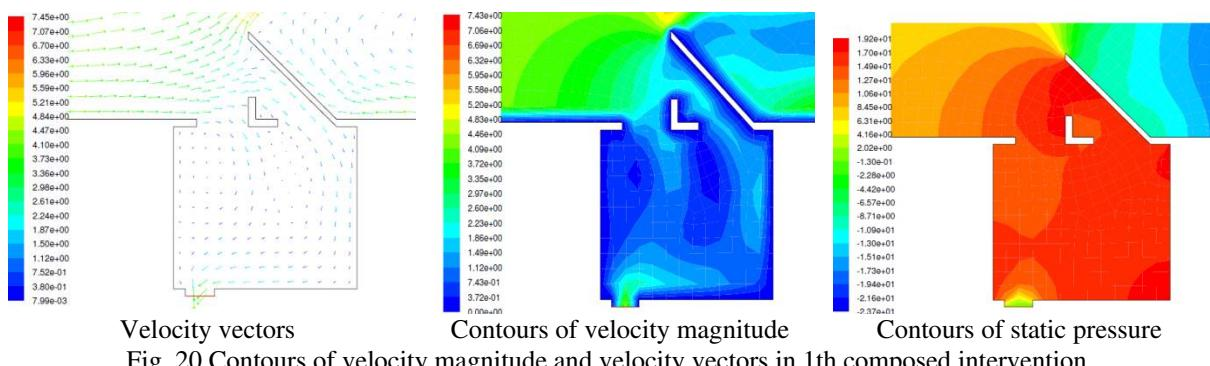
Fig. 20 Contours of velocity magnitude and velocity vectors in 1th composed intervention
