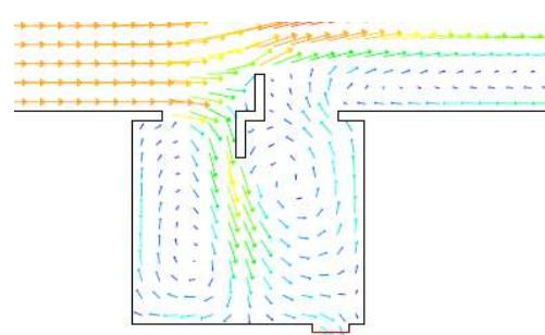
Fig. 16 Velocity vectors in 6th intervention
