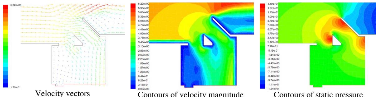
Fig. 23 Contours of velocity magnitude and velocity vectors in 4th composed intervention
