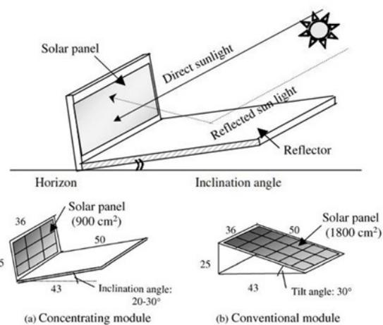
**Fig.1. Position of PV panel relative to the flat mirror and the Sun (up). Comparison of slope angle and the area of the solar panel combined with reflector (down-left) with one without reflector (down-right)**
