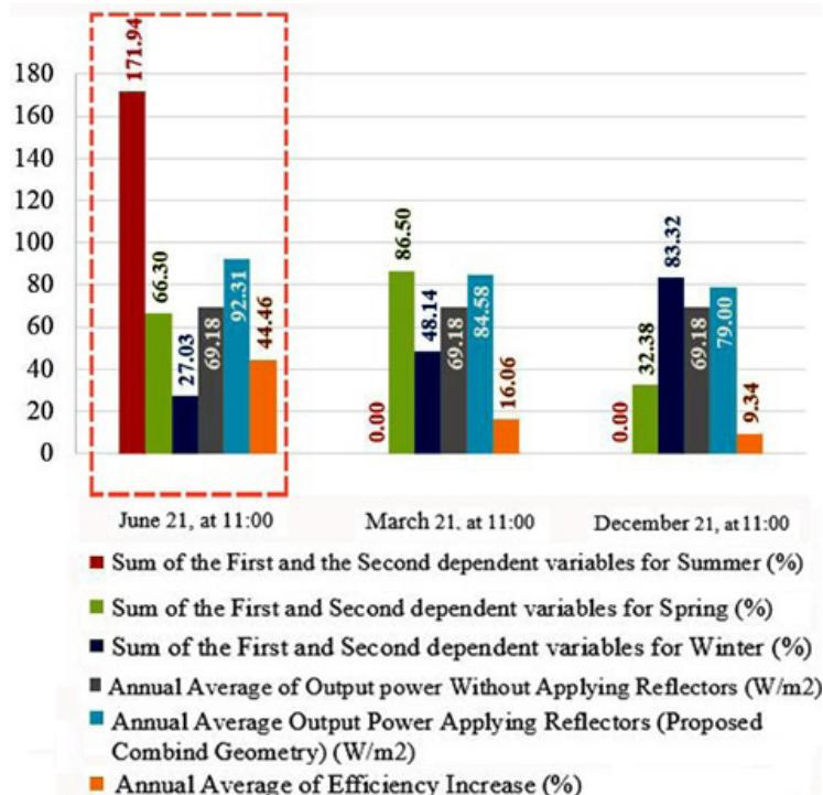
Fig.13. Annual output comparison when the algorithm is adjusted according to the optimum answer of each season (the first and the second dependent variables are “Increase in Radiation” and “Area of Reflections/ Panels area” respectively)
