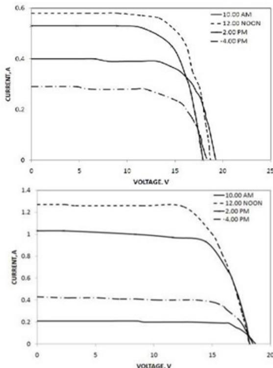
Fig.2. Combination of flat reflectors and the PV panel (up), Voltage-Current characteristic without using reflectors (middle) and applying 4 flat mirrors (down). ( Sathyanarayana, Ballal, kumar, & Laksmi sagar, 2014, pp. 358,360)
