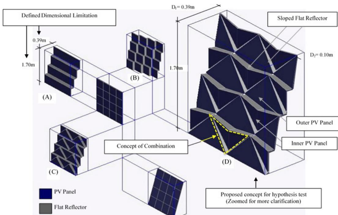
Fig.7. Various alternations of combining flat reflectors and PV panels in defined dimensional limitations: (a) Just using horizontal mirrors, (b) Using horizontal and vertical mirrors, (c) Using horizontal and sloped mirrors and (d) Just using sloped mirrors.(Concept of combining reflectors and PVs, which shapes the form of the proposed envelope, has been shown)
