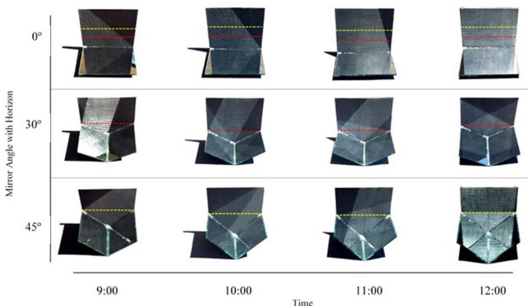
Fig.5. Reflection of a flat mirror on a given vertical plate while the angle of reflector varies from  $0^{\circ}$ - $45^{\circ}$  on June 22, from 9:00 to 12:00. The red and yellow lines show the equivalent level of enclosed space between  $30^{\circ}$  and  $45^{\circ}$ -sloped mirrors respectively
