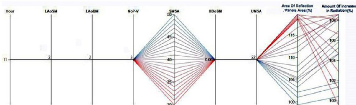
Fig.16. The effect of change in SMSA amounts on the dependent variables (Black columns represent input parameters and the blue ones show the outputs or dependent variables; each continuous line stands for one change in SMSA amount).
