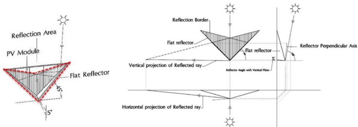
Fig.6. Using of triangle flat reflector for casting reflection as a combination concept (left) and drawing the reflection of a two  $45^{\circ}$ -sloped flat reflector with the lateral angle of  $5^{\circ}$  under the sun radiation on June 22, at noon (right).
