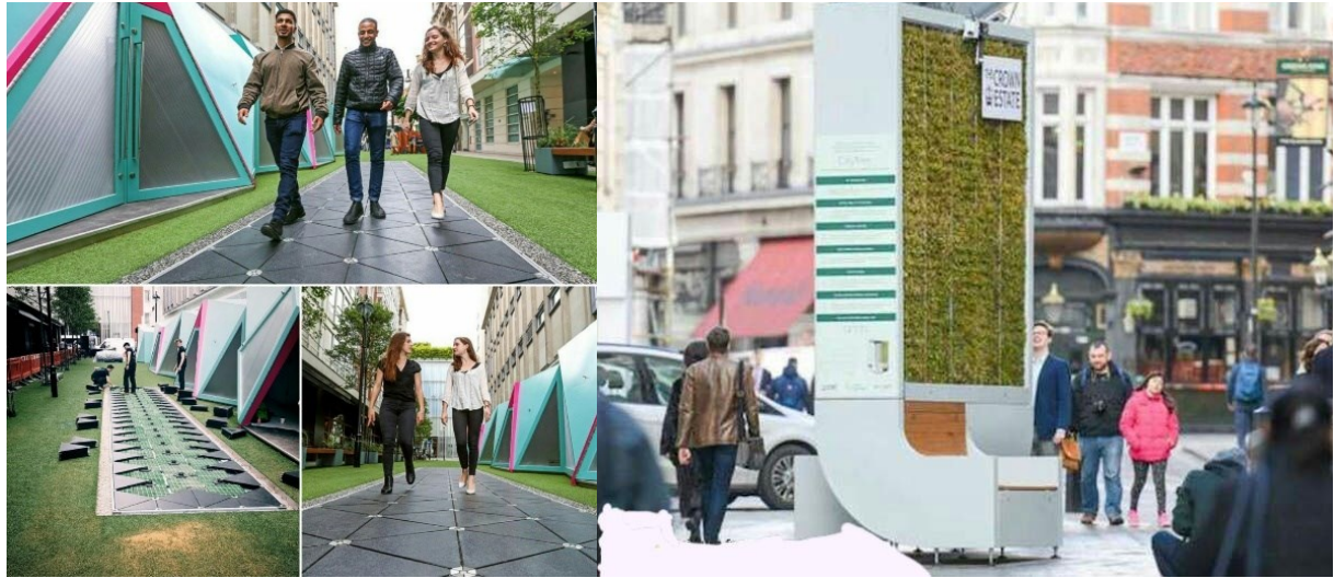
Fig. 1. Intelligent environment in an urban space where sidewalk flooring converts mechanical energy of pedestrians to electrical energy
