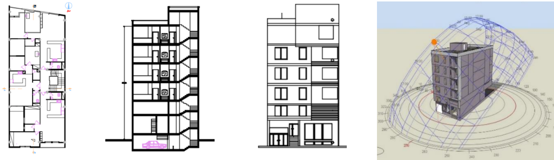
Fig. 7. Specifications of the selected building in Bushehr, from left to right: 1. Floor plan; 2. A-A section; 3. North view; 4. 3D simulation
