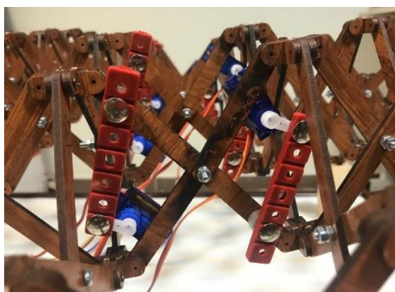
Fig. 9. Connection of servo-motors to Akgun M-SLEs
