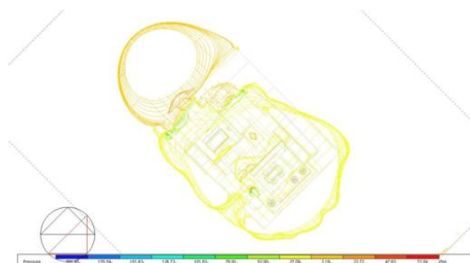
Fig. 7. Simulation of effective pressure due to wind on Golshan House (plan)
