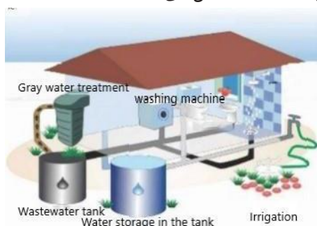
Fig. 4. Establishing a treatment center near the site and using treated wastewater for irrigation
